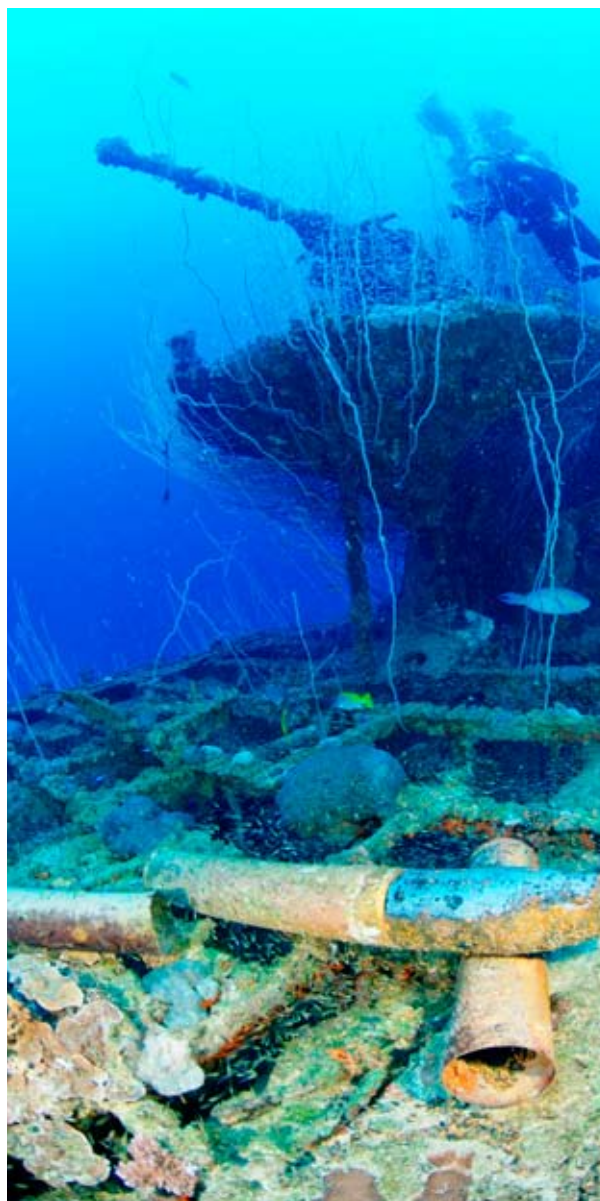
Figure 51. Divers on the Apogon conning tower. The ships at Bikini Atoll appear to demonstrate accelerated corrosion as a result of the atomic tests (E. Hanauer, 2006)
